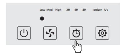
When the "Speed" indicator is flashing, this indicates that the installed filters are coming to the end of their useful life and should be replaced.
