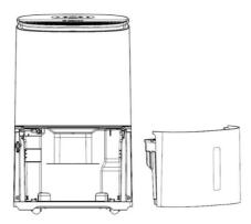
Step 1: Remove the water tank.
