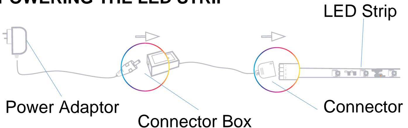
Connect the connector box to the LED strip, ensuring the arrow on the connector is to the left of the strip. Then connect the power adaptor to the connector box, before plugging into a wall socket.
