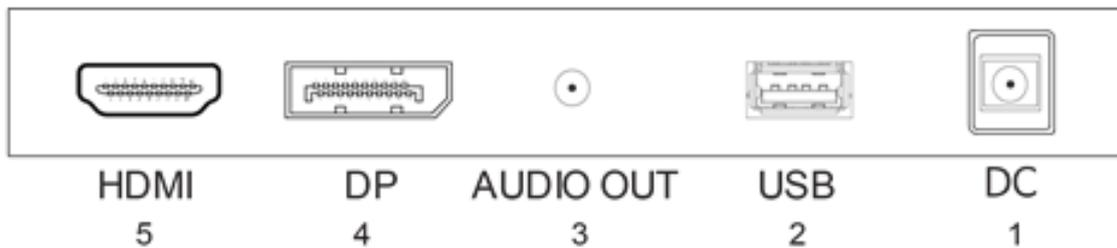
1. DC input port: Connect the supplied power supply to power the monitor
