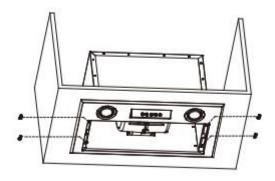
Screw the stainless steel frame back into place using the 4 screws removed as described above.
