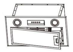
Press the lock catch of metal Filter, remove the Filter.
