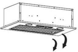
Activated carbon filter can be used to trap odors. Normally the activated carbon filter should be changed at three or six months according to your cooking habit. The installation procedure of activated carbon filter is as below.
