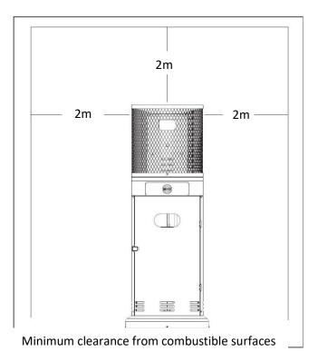
**DO NOT** operate this heater unless it is fully assembled. Respect the minimum clearances from combustible materials.
