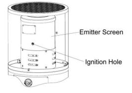
Note: it is possible to light the appliance using a long match by lighting the burner through the ignition hole in the emitter screen.
