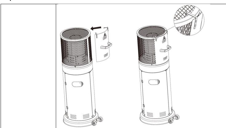
Clip the heat cover onto the Burning System Assembly. Use the handle to slide the heat cover around the mesh to block heat from that particular section.
