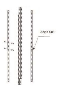
2. Calculate the length of the angle bars according to the overall height of the hood required. Extend the angle bars to the required height and then fix them in position using the 16 x M5 screws. The angle bars must have an overlap of at least 100mm.
