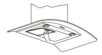
Put the activated carbon filter onto the end of the motor unit and turn it in clockwise direction. Repeat the same on the other side (see diagram)
