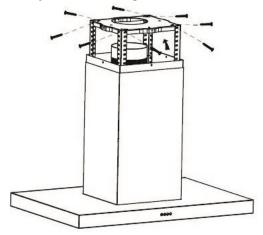
**IMPORTANT**: This stage of the installation process MUST be completed by two people, as one person must support the weight of the hood until all the screws have been securely tightened.
