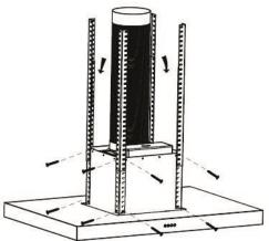
5. Slide the inner chimney and outer chimney onto the angle bars.
