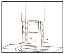
6. Lift the main body of the cooker hood onto the angle bar and then fix it into position using the 16 x M5 screws.
