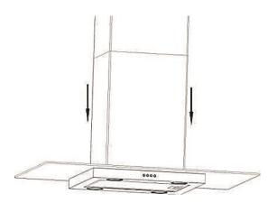
7. If externally venting, connect the exhaust pipe to the hanging plate.
