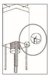
4. At this point, if the unit is to be externally vented connect the ducting hose to the hanging plate. Then fix the upper chimney section to the hanging plate, using the 4 x self-tapping screws (4mm x 6mm).
