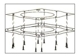
Please ensure that the bracket is fixed in a way it would support the weight of the hood. Depending on the construction of the ceiling, alternative fixings may be required. 6 x expansion bolts are also provided to allow fitting to concrete.
