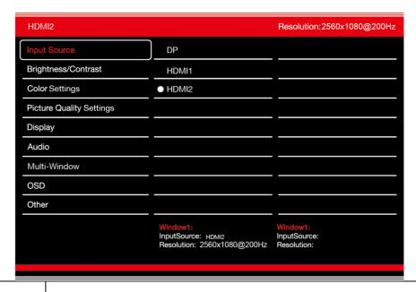
Signal Switch the signal input or select the source. DP, HDMI1, HDMI2
