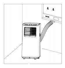
Fix the end of the fishtail to the air-outlet window kit.
