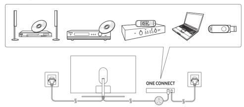
You can connect various external devices using the connectors located at the back of the product. Check the connectors and then refer to the Quick Guide for more instructions on supported external devices.
