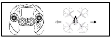
If the drone drifts left, tap the Right Directional Trim button until the drifting stops. If it drifts right, the Left Directional Trim Button should be pressed until drifting stops
