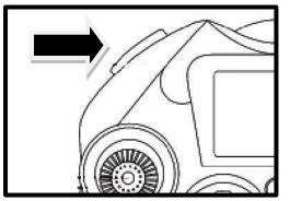
The aircraft can be made to return in a fixed direction by pressing and holding the return button for 3 seconds. When the aircraft is turned on it will remember the direction it is oriented and upon activation of the Smart Return feature it will fly back in that direction.
