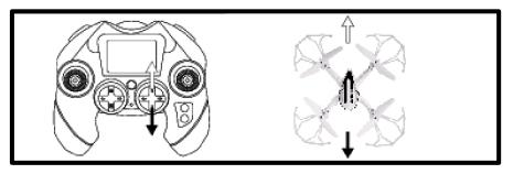
If the drone drifts forward, tap the Down Directional Trim button until the drifting stops. If it drifts backwards, the Up Directional Trim Button should be pressed until drifting stops
