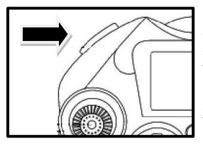
Both drones are equipped with IR Laser emitters which enables you to fire at your opponent while flying. The Laser can be fired by pressing the left Fire button. The range is around 10 feet, and shoots out at an angle of 45 degrees from the front of the drone.
