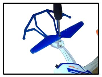
Using a screwdriver, untighten the screw holding the propeller in place and remove the propeller. Insert the new propeller over the motor spindle and use a screwdriver to tighten the screw.
