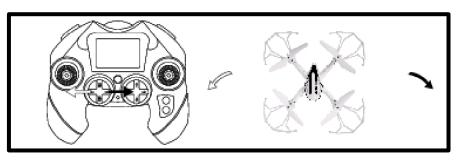
If the drone spins anti clockwise, tap the Right Directional Trim button until the drifting stops. If it spins clockwise, the Left Directional Trim Button should be pressed until drifting stops
