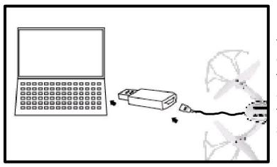
Unplug the battery cable from the socket in the back of the drone, and connect the cable to the supplied USB charging adaptor. The adaptor should then be plugged into a usb socket to charge
