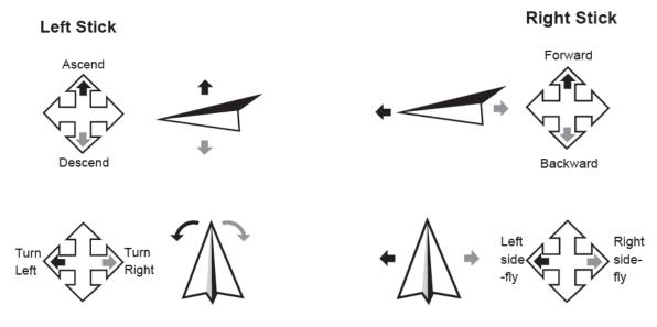
The aircraft can only take off and land by pressing the take off / land button (click once to take off and once to land). Once the aircraft is airborne it will hold a steady hover, you are now in control of the aircraft and can use the left and right sticks to control it.
