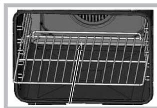
**!** When inserting the shelf make sure the backstop is at the rear of the cavity (see image)
