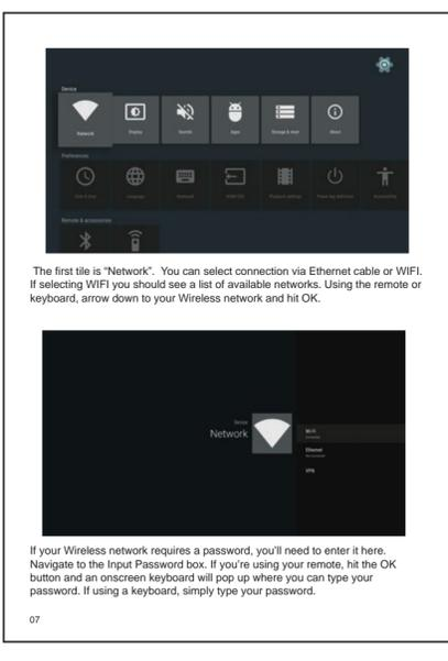
The first tile is "Network". You can select connection via Ethernet cable or WIFI. If selecting WIFI you should see a list of available networks. Using the remote or keyboard, arrow down to your Wireless network and hit OK.
