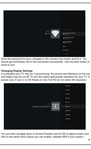
Once the password is input, navigate to the connect now button and hit it. You should get verification that it has connected successfully. Use the back button or home to exit.
