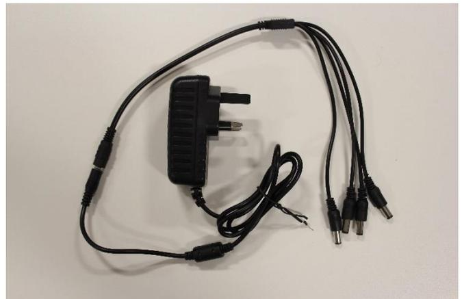
(1) Attach one of the 4 ends from the multiplexer to the red power lead, which is connected to a camera.
