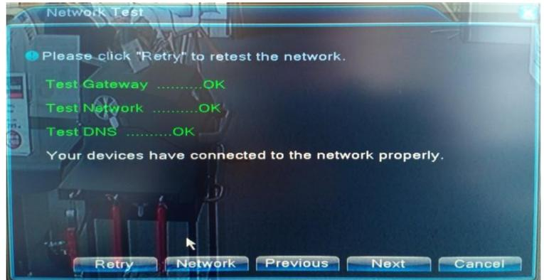
If any state ERR in red, the network settings need to be changed to connect successfully to the network. To do this click on the network button at the bottom to view the network settings
