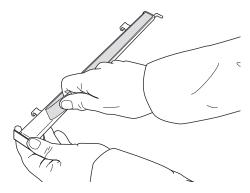
**3.** Fasten the upper clip of the runner to the shelf guide and slide it along as far as it will go. (fig. A); lower the other clip into position.
