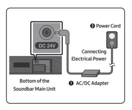
• Make sure to rest the AC/DC Adapter flat on a table or the floor. If you place the AC/DC Adapter so that it is hanging with the AC cord input facing upwards, water or other foreign substances could enter the Adapter and cause the Adapter to malfunction.
