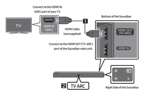
1. With the Soundbar and TV turned on, connect the HDMI cable (not supplied) as shown in the figure.
