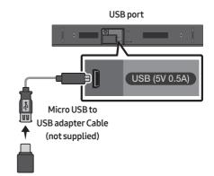
If an update is offered, you can update the firmware by connecting a USB device with the firmware update stored on it to the USB port on your Soundbar.
