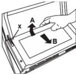
You must remove the oven door glass before cleaning. Push the glass in the direction of B and release from the location bracket (x). Pull the glass out in the direction of A.
