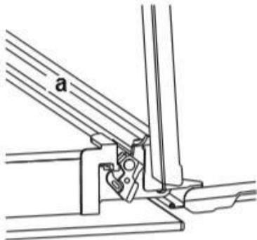
Open the oven door and open the locking catch (a) with a screwdriver, turning anti-clockwise. Begin to close the door until it is almost closed, and then lift the door up to remove it.
