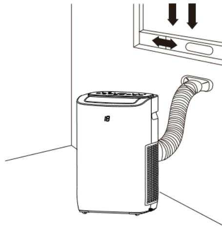
3. Partially open the window and place the extended slide bar in position before closing the window onto it.
