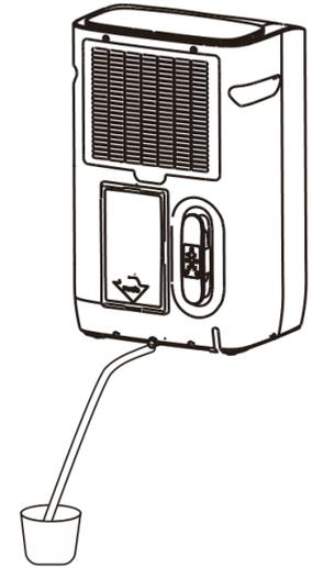
**NOTE:** This model has a self-evaporative function, which reduces the need to empty the water tank in cooling mode. If the unit is vented correctly most of the water is reused to cool the condenser coils and any excess is evaporated. Please do not use continuous drainage if you intend to use the self-evaporating facility.
