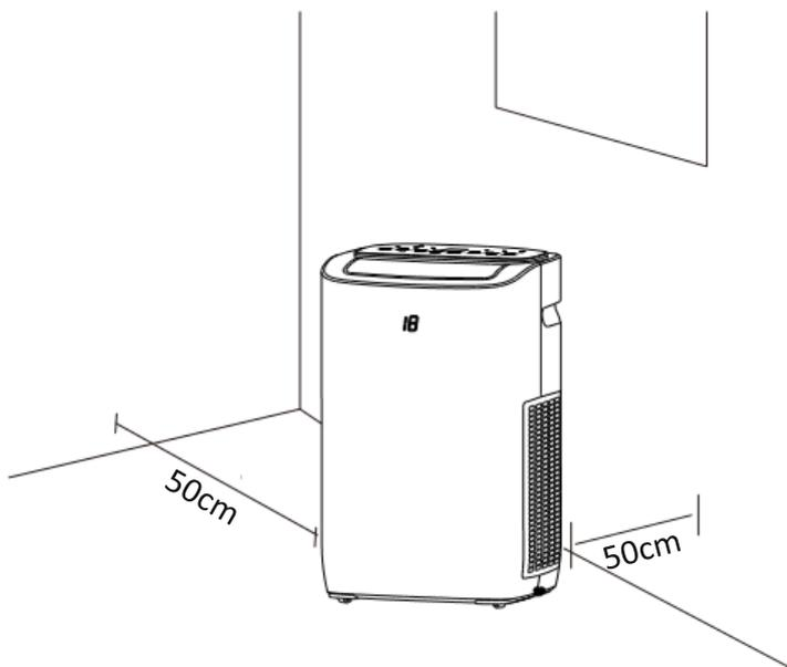
4. Make sure the unit is upright and there are no obstructions to the air inlets and outlet grills, with at least 50cm of space to the sides and rear of the unit.
