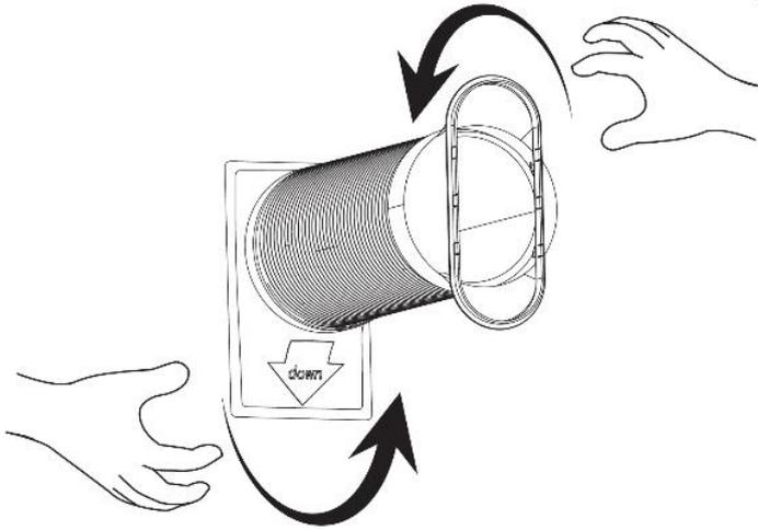
1. Attach the fishtail connector to the end of the hose, by extending the end of the hose and twisting until firmly attached to the connector (At least 3 full rotations).
