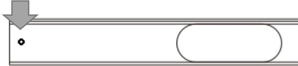
2. Slide the rear section of the slide bar onto the front section lining up the plate so it runs within the groove. Extend the bar to the required length, and use the supplied wing nut to secure
