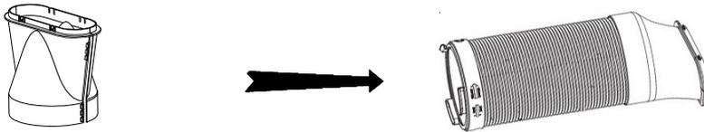
2. Extend one head of the hose and screw it into the unit anti-clockwise.
