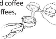
Fill the filter a little at a time to prevent the ground coffee from overflowing.
