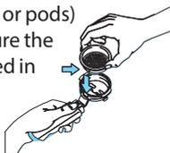
**3. INSERT A POD**, centring it as far as possible on the filter. Always follow the instructions on the pod pack to position the pod on the filter correctly.
