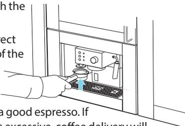
**4. REMOVE ANY EXCESS COFFEE** from the rim of the filter holder and attach the filter holder to the appliance.
