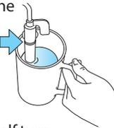
**6. WHEN THE REQUIRED TEMPERATURE IS REACHED (60°C is ideal),** interrupt steam delivery by rotating the steam knob clockwise and at the same time pressing the steam button.
