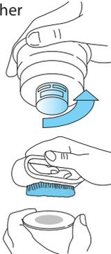
**MAKE SURE** the holes in the metal filter are not blocked. If necessary, clean with a pin.
