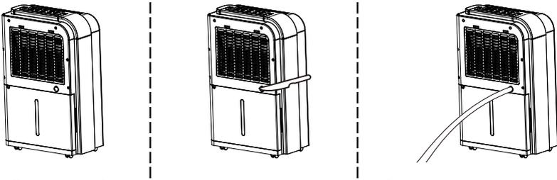
1. Cut off the cover for the continuous drain on the back of the unit.
