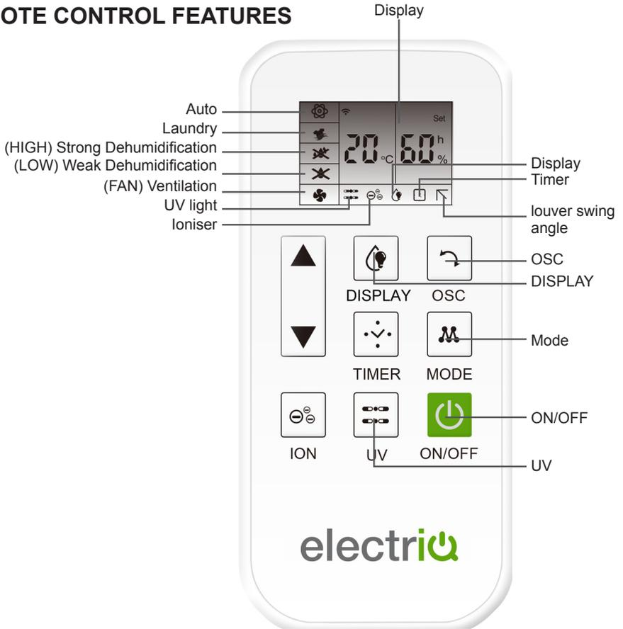
As well as containing an independent humidistat, allowing the humidity of the room to be measured away from the dehumidifier, the remote control contains many of the same buttons as found on the main unit, as well as a few other features.
