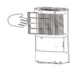
**1. CLEAN THE GRILLE AND CASE** Use water and a mild detergent to clean the washable mesh filters. Do not use bleach or abrasives. Do not splash water directly onto the main unit. Doing
