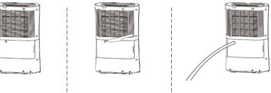
Make sure the connection between pipe and the drain outlet is tight and does not leak. Then direct the pipe to a suitable drainage point. This unit uses gravity to dispose of water hence the drain should be lower than the water outlet on the unit. Put the tank back. Be sure to run the water pipe downward and let the water to flow out smoothly. Do not kink or bend the pipe.
