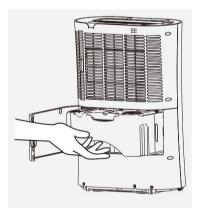
**NOTE:** When you remove the water tank, do not touch sensors or any parts which are situated behind tank. Doing so may damage the product. Be sure to push the tank gently all the way into the unit. Banging the bucket against anything or failing to push it in securely into place may cause the unit not to operate.
