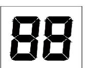
**Notes:** When humidity level is outside the normal operational parameters will show LO/Hi. If ambient humidity is lower than 20%, it will show "LO" If ambient humidity is higher than 90%, it will show "HI"
