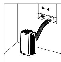
**Note:** The window kit is only designed to be installed with sliding or sash windows or doors. The window kit is not designed or to be used with any other style of windows.
