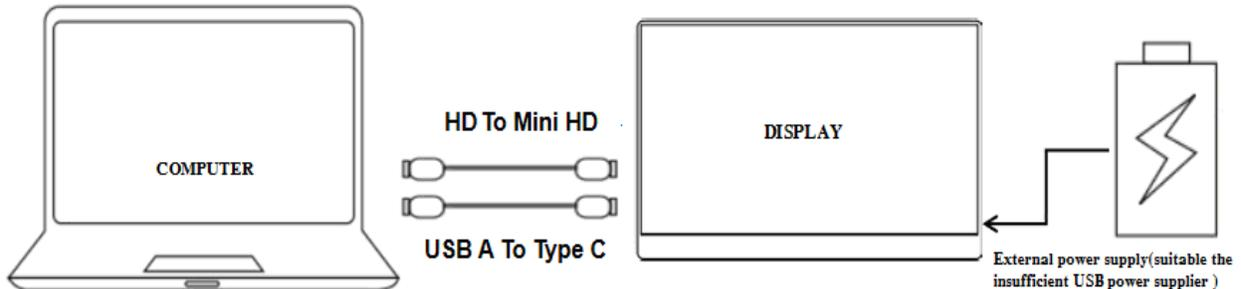
When connecting to a compatible computer using the HDMI interface, you need to connect the supplied HDMI cable between the computer and the display. You should also connect the display to the computer via USB, using a USB to USB Type C cable (Not supplied), connected to the left-hand Main USB Type C socket on the left of the display.
