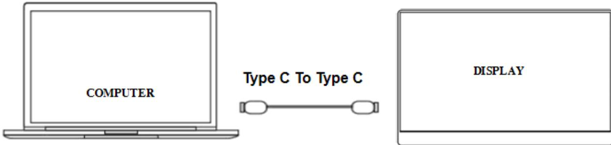
The portable display can be connected to a compatible computer using the supplied USB C cable. This must be connected to the Main USB socket on the left of the display. The computer will provide power and signal to the monitor and can be used for extended display or duplicated display use.
