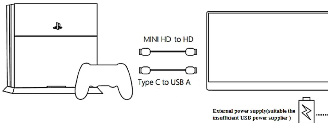
When connecting a device using HDMI, be sure to connect the power cable first, then connect the HDMI to ensure the smooth transmission of the signal.
