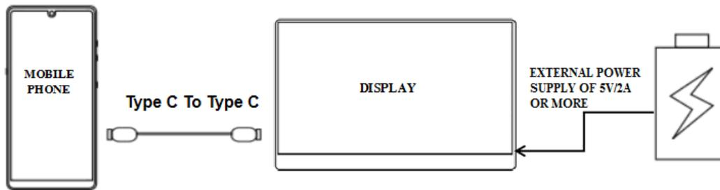
When there is no external power supply connected to the secondary USB Type C socket on the right of the display, the mobile phone battery will supply power to the display. To reduce power usage the energy-saving mode will be activated and the display brightness will be reduced to 30%, and the user can adjust the brightness and volume of the display according to the output power of the mobile phone).
