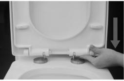
4. Try the seat on the hinges, re-adjust it if the distance does not match until it fits. Take off the metal cover and tighten the screws
