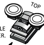
TURN ADJUSTER SCREW UNTIL THERE IS AN EQUAL GAP BEFORE FITTING.
