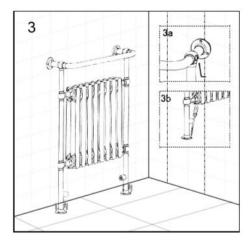
4. Insert the air vent in the top of the radiator, (add a little sealer tape to secure) and tighten, be sure not to overtighten then fit the radiator valves to the pipework and connect to the radiator valve tail and tighten all connections.
