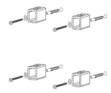
**Please note:** If drilling into a tile, it is recommended to tape the wall to prevent the drill from slipping.
