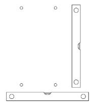
3. Using the drill and 8mm drill bit, drill into the marked positions then insert the wall plugs and tap flush to the finished wall surface. Next, position the wall brackets and screw into place using the screws provided (securing each with a washer) with the Philips screwdriver.
