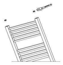
Mark the position of the wall brackets (on the wall) approximately 5cm in from the inner edge of the towel radiator vertical bar. Use a spirit level to ensure that these are aligned.
