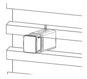
6. Finally, fit the radiator valves to the pipework and connect to the radiator valve tail and tighten all connections.
