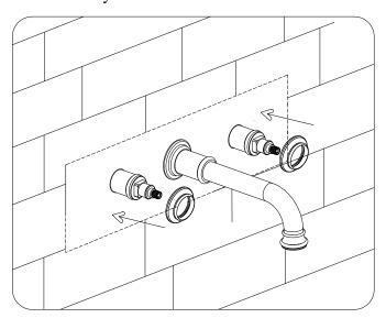
Install the lever handles and ajdust to the correct positions. Securing them with the grub screw and then fix the ceramic cap.
