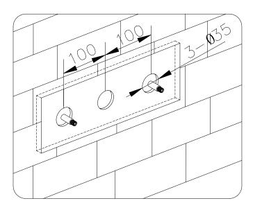
Fix the decorative base onto the spout. Install the spout using thread seal tape.
