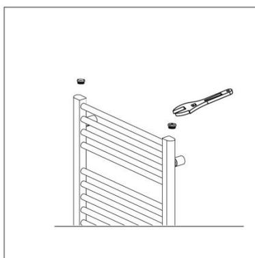
2. The rear of the towel rail has four location holes to fix the brackets. Measure the distance between all the location holes and mark these on the wall in the required location, use a spirit level to ensure these are horizontally and vertically aligned.
