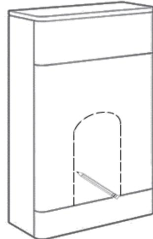
Mark these dimensions on to the front panel of the unit using a pencil
