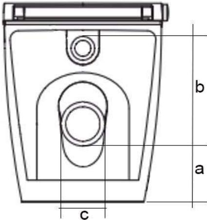
Measure the height from the floor to height a then measure height b and allow 5mm tolerance, then measure width c and allow 5mm
