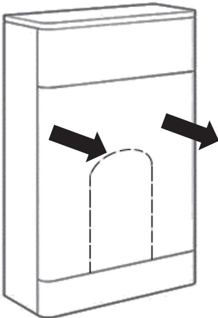
Remove the front panel from the unit and cut the hole to allow the waste pipe and flush pipe to pass from the cistern
