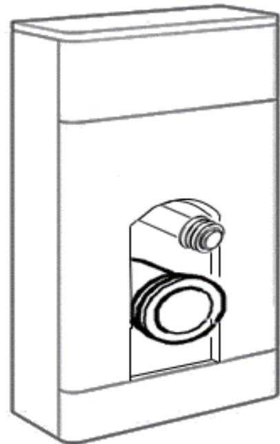
It is recommended to seal the cut edge and bottom edge of the unit, to protect against moisture ingress
