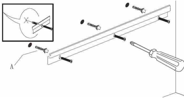
6. Place the hanging bar back onto the wall, lining up the 3 holes with the wall plugs.
