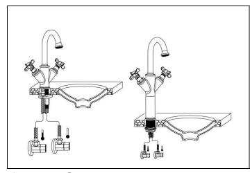
Check the washers are fitted into the nut on the hot and cold flexible hoses.
