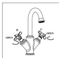
Hot valve(H): open by turning clockwise, close by turnning counterclockwise;
