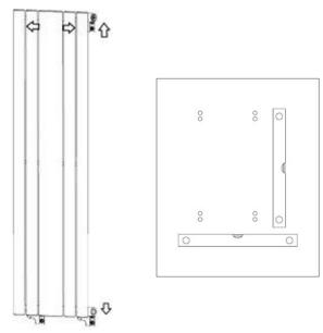
3. Using the drill and 8mm drill bit, drill into the marked positions then insert the wall plugs and tap flush to the finished wall surface.
