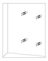
**Please note:** If drilling into tile, it is recommended to tape the wall to prevent the drill from slipping.
