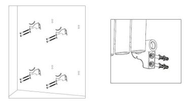
5. Once all brackets are secure, hang the radiator until fixed firmly into place and adjust so that the radiator aligns with the pipework.
