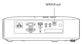
Use a USB cable with a micro USB plug on one end for connection to the projector's SERVICE port, and a plug on the other end with a shape that is compatible with the computer USB port.
