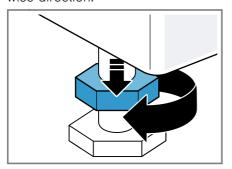
2. To align the appliance, turn the appliance feet. Check that the appliance is level using a spirit level.
