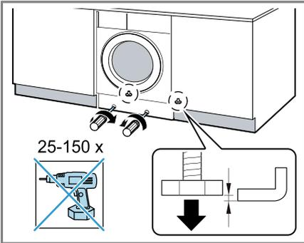
8. Align the appliance using a spirit level.
