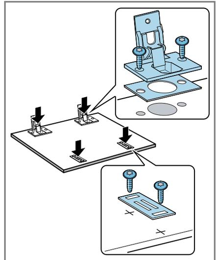
5. Screw on the counter plates for the magnetic catches.
