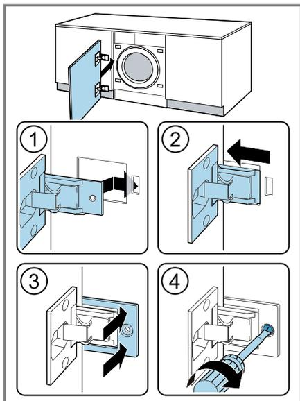
7. Slide in the covering rail ③ and screw it in ④.
