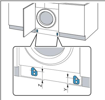
3. Screw the spacers in as per the dimensions.
