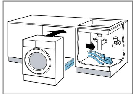
5. Connect the water inlet hose. Connecting the water inlet hose
