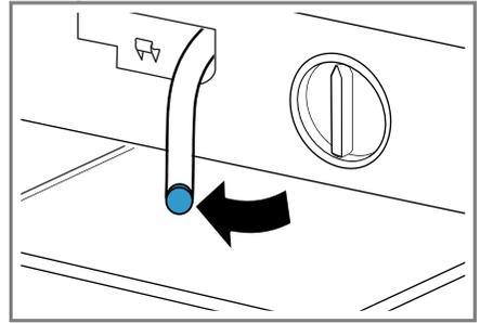
9. Insert the drain hose into the holder.
