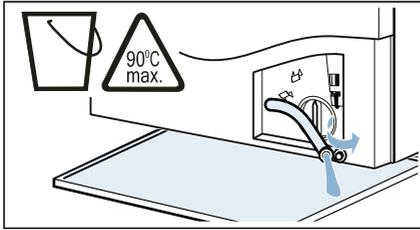
4. Carefully unscrew the pump cover; residual water may leak out.
