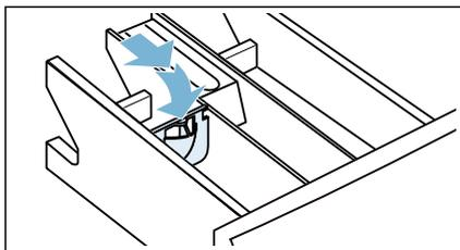
**Note:** Do not use the measuring aid for gel detergents and washing powder, or for programmes with pretreat when "Finish in" time is selected.
