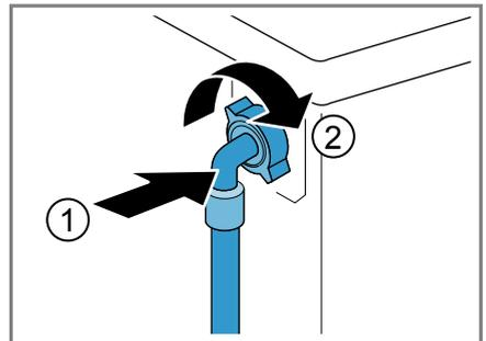
2. Connect the water inlet hose to a tap (26.4 mm = 3/4").
