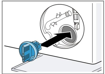
5. Screw on the pump cap.
