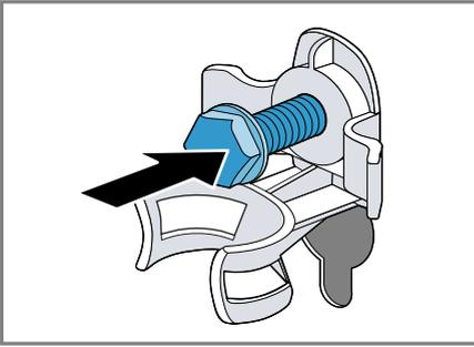
4. Insert the power cord into the holder ① and tighten all four screws for the transit bolts with a WAF 13 wrench ②.
