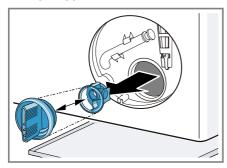
Clean the interior, the thread on the pump cap and the pump housing.
