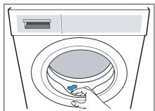
Leave the door and detergent drawer open so that residual water can evaporate.
