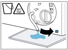
9. Firmly press on the sealing cap.
