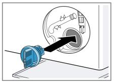
5. Screw on the pump cap.
