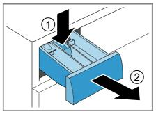
3. Pull out the insert upwards.
