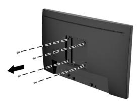
Install the mounting plate to the wall or swing arm of your choice using the four screws that were removed from the VESA holes on the rear of the display head.
