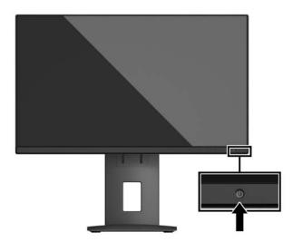
CAUTION: Burn-in image damage may occur on monitors that display the same static image on the screen for 12 or more consecutive hours of nonuse. To avoid burn-in image damage on the monitor screen, you should always activate a screen saver application or turn off the monitor when it is not in use for a prolonged period of time. Image retention is a condition that may occur on all LCD screens. Monitors with a "burned-in image" are not covered under the HP warranty.
