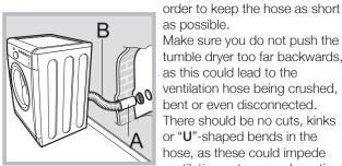
as possible. Make sure you do not push the tumble drver too far backwards. as this could lead to the ventilation hose being crushed, bent or even disconnected. There should be no cuts, kinks or "U"-shaped bends in the hose, as these could impede
