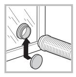
towards the air inlet pipe on the rear of the appliance. The ventilation hose must always be fitted to ensure optimum performance. Make sure that the ventilation hose and the air inlet vents are not obstructed or blocked. Do not let the tumble drver recirculate exhaust air. Improper use of the tumble
