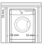
air inlets on the rear panel are not blocked or obstructed.
