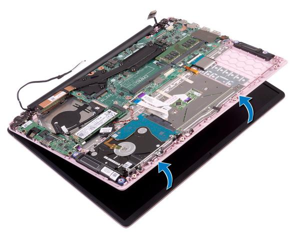
h Lift the display assembly away from the palm-rest and keyboard assembly.
