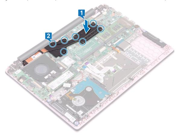
For the systems shipped with UMA model, align and place the heatsink to the slot on the system board and then tighten the four captive screws in sequential order as indicated on the heatsink to secure the heatsink to the system board [1, 2].
