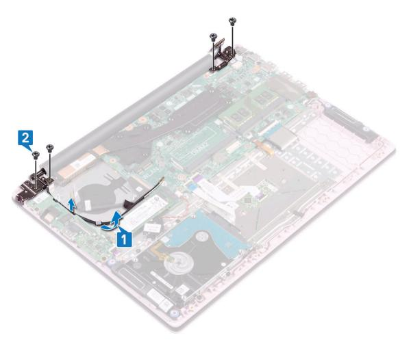
g Open the display assembly at an angle of 90 degrees.
