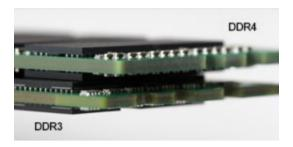
Figure 2. Thickness difference
