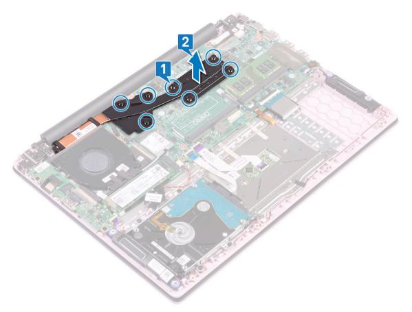
c For the systems shipped with UMA model, loosen the four captive screws in sequential order (as indicated on the heatsink) that secure the heatsink to the system board and lift the heatsink away from the system [1, 2].
