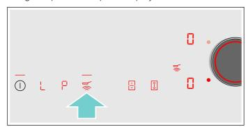
**2.** Within the next 5 seconds, select the required temperature setting using the twist knob.
