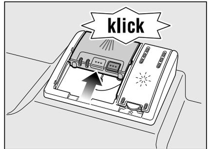
The detergent dispenser opens automatically at the optimum time depending on the programme. The powder or liquid detergent is distributed in the appliance and is dissolved. The tablet falls into the appliance and dissolves.
