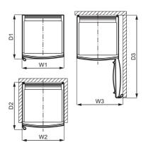
the cooling air, plus the space necessary to allow door opening to the minimum angle permitting removal of all internal equipment
